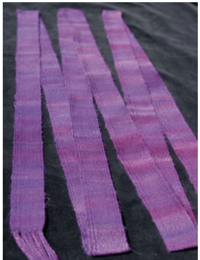
Right: The finished binding, 2.4 m at 30 picks per cm (75 picks per inch), weft faced cloth
